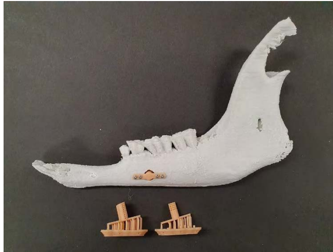
The above image is the customised 3D printed PEEK bone implants.
